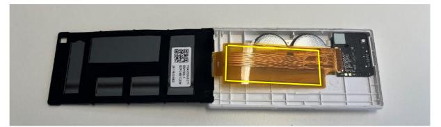
(Explanation: In the illustration, the area in which the antenna is attached to the rear of the foil is marked in yellow by the court; the "upper area" (section) of the rear housing surface can be seen in the illustration *below*; the lower section of the rear housing surface (battery compartment and black circuit board) is molded deeper than the area above it in view of the arrangement of the batteries and the circuit board)
